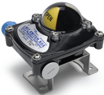
Inductive limit switch for visual and electric indication of actuator position voltage: 8V DC, Enclosure IP67
